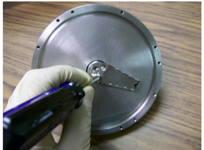
Step 9: Remove 2 each #8-32 x 1/4 Flat Head Philips screws
