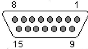
I/O connector DB15F (socket) connection (viewed from back panel)
